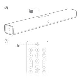
Follow the same procedure for VOLUME - and VOLUME +. For mute, press both VOLUME + and VOLUME - button on soundbar and press MUTE button on TV remote control. Press and hold VOLUME+ and SOURCE button on soundbar again for 5 seconds and now your soundbar responds to your TV remote control\*.
