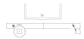
Screw the wall mount brackets on the pen mark; screw the threaded mounting post into the back of the soundbar; then hook the soundbar on the wall.
